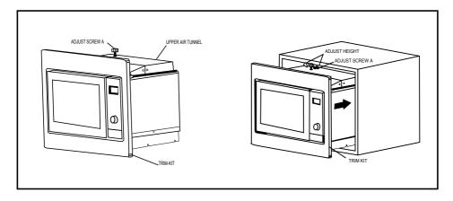
1. Fix ADJSUTSCREW A on the UPPER AIR TUNNEL of the oven, and then install the oven into the cabinet.
